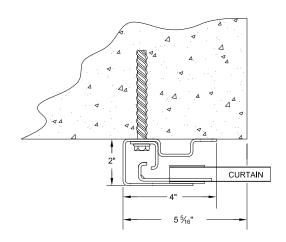
CONCRETE/FILLED BLOCK JAMBS USING 3/8" X 4" POWERS WEDGE BOLT
