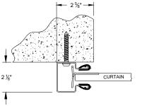
CONCRETE/FILLED BLOCK JAMBS (USING  $\frac{5}{16}$ " X 2  $\frac{7}{4}$ " TAPCON XL) OR (DEWALT ULTRACON)
