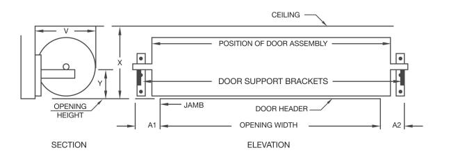
CEILING: LOCATE DIMENSIONS AND CLEARANCE ON DIMENSION PANEL. STANDING ON THE INSIDE FACING OUT. DRIVE TYPE IS ON RIGHT SIDE UNLESS OTHERWISE SPECIFIED.
