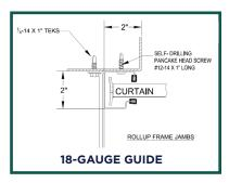
Universal mount 2" deep, 18-gauge galvanized steel guides require no pre-installation modifications for wood, steel, concrete or filled masonry block applications.
