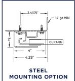
Steel mounting options are limited to the option shown above. Wood and filled block mounting options are not pictured.
