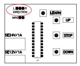
All "mini" logic controllers shall have the jumper positioned as shown on the JSS(MINI) terminal.
