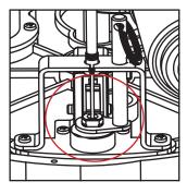
Reinstall knurled split nut and tighten.
