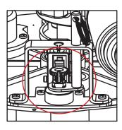
Pull ring on spring loaded pin and twist to disengage auto (electric) mode.
