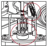
Uncoil the manual release cable and insert the free end of the cable into the threaded recess where the knurled split nut was removed.
