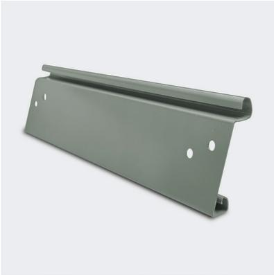
**SLAT PROFILE:** Manufactured from commercial-grade galvanized steel and coated with super durable polyester paint backed by a 40-year film integrity and 25-year no-fade paint warranty. Injected polyurethane foam, effective insulating value to be R=7.2.
