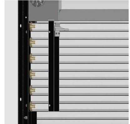
**GUIDES:** Angles to be 3/16" minimum thickness structural steel with removable head stops and 30" service cut-out. Guide depth to provide slat penetration adequate to satisfy specified windloading.
