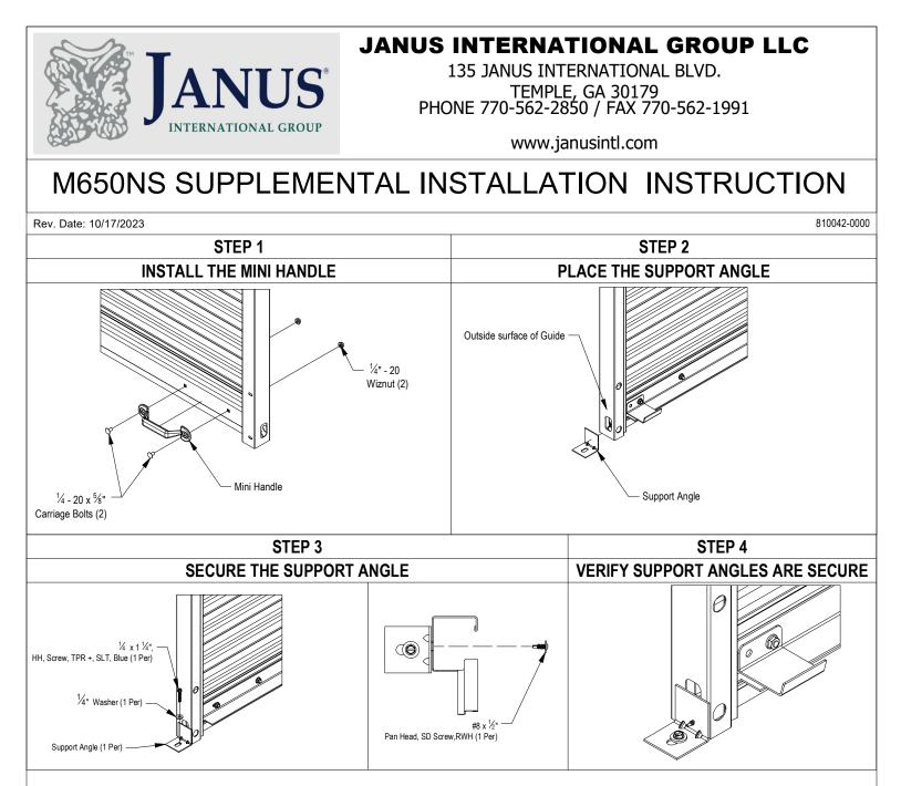
STEP 1: Install the Mini Handle to the bottom bar on latch side of door using (2) <sup>1</sup>/<sub>4</sub>" - 20 x <sup>5</sup>/<sub>8</sub>" Carriage bolts and (2) <sup>1</sup>/<sub>4</sub>"-20 Wiznuts.
