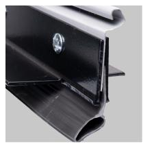
**BOTTOM BAR:** Curtain bottoms are reinforced with a bottom bar consisting of 2 structural steel angles with PVC bulb astragal for maximum durability.
