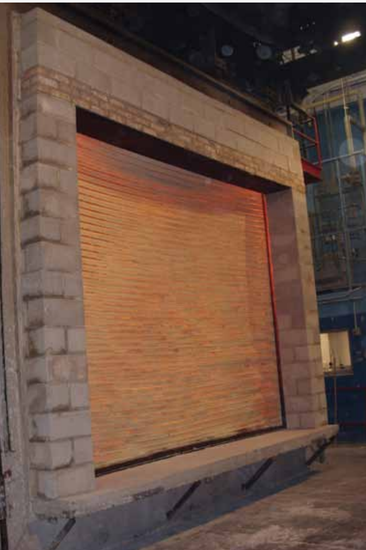
A Sure-Set™ fire door undergoing a 4 hour endurance burn test.
